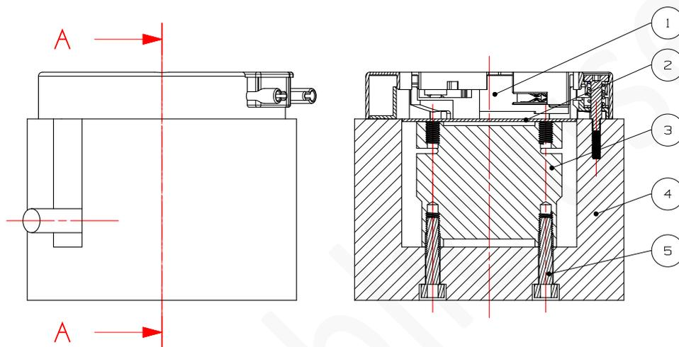
**Figure A-20 : Assembly of mounting platform, force transducer and Holder under test**
