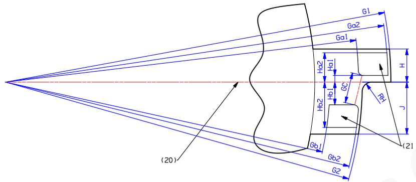
Figure 3-3: Base electrical contact definition
