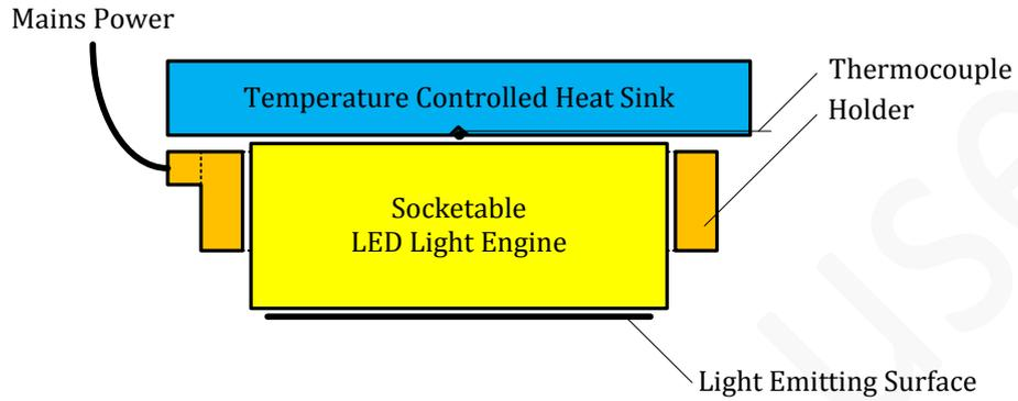
**Figure A-8: Definition of Test Fixture OETF-PHJ65d-x**
