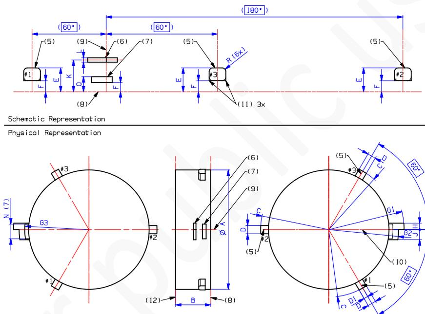
Figure 3-2: Dimensions of the Base
