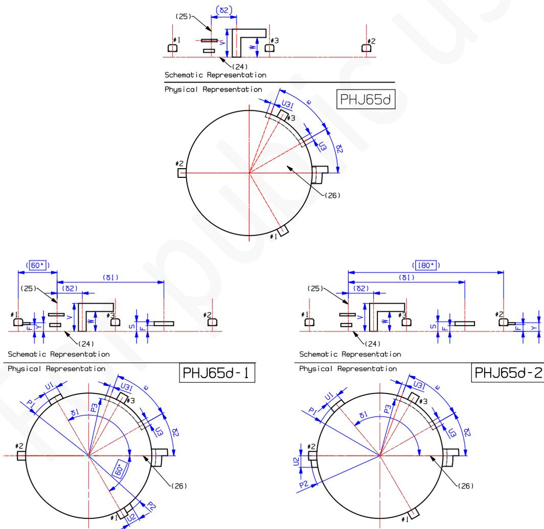
Figure 3-4: Base mechanical fit Keying definition (top view)
