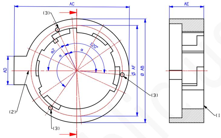
Figure 3-5: Maximum outline of a Holder (bottom view on the left)
