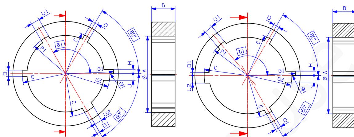
Figure A-1: Dimensions of MTG-B1 (left) and MTG-B2 (right)
