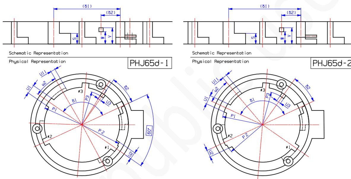
**Figure 3-8: Holder mechanical fit Keying definition (top view)**
