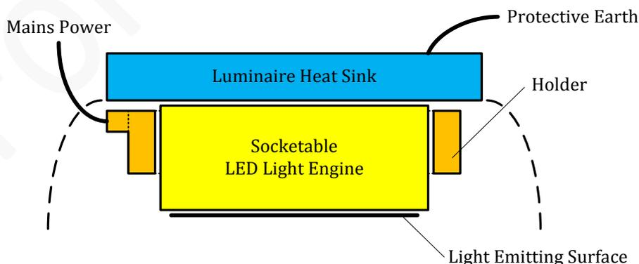
Figure 2-1: Schematic view of the assembly of a Socketable LLE, Holder and Luminaire
