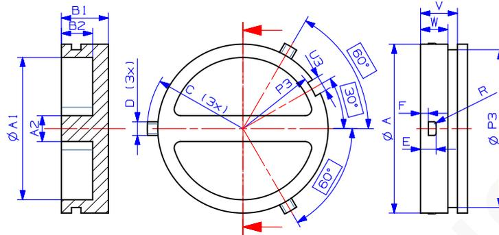
**Figure A-18 : Dimensions of MFG type A and type B**
