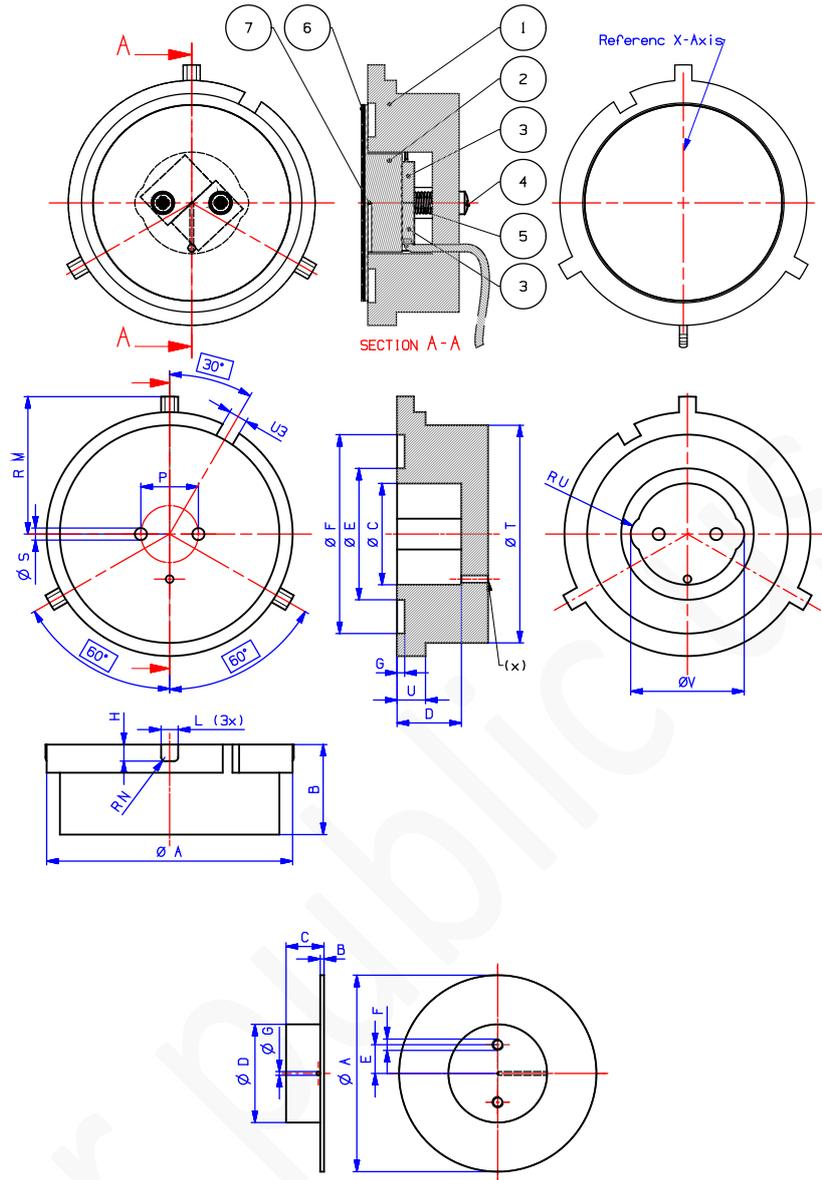
Figure A-22: Thermal Test Engine TTE-PHJ65d — force inducer (top) and power inducer (bottom)
