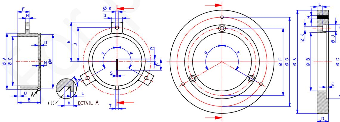
**Figure A-10: Test Fixture TUTF-PHJ65d-x — heat sink (left) and mounting ring (right)**
