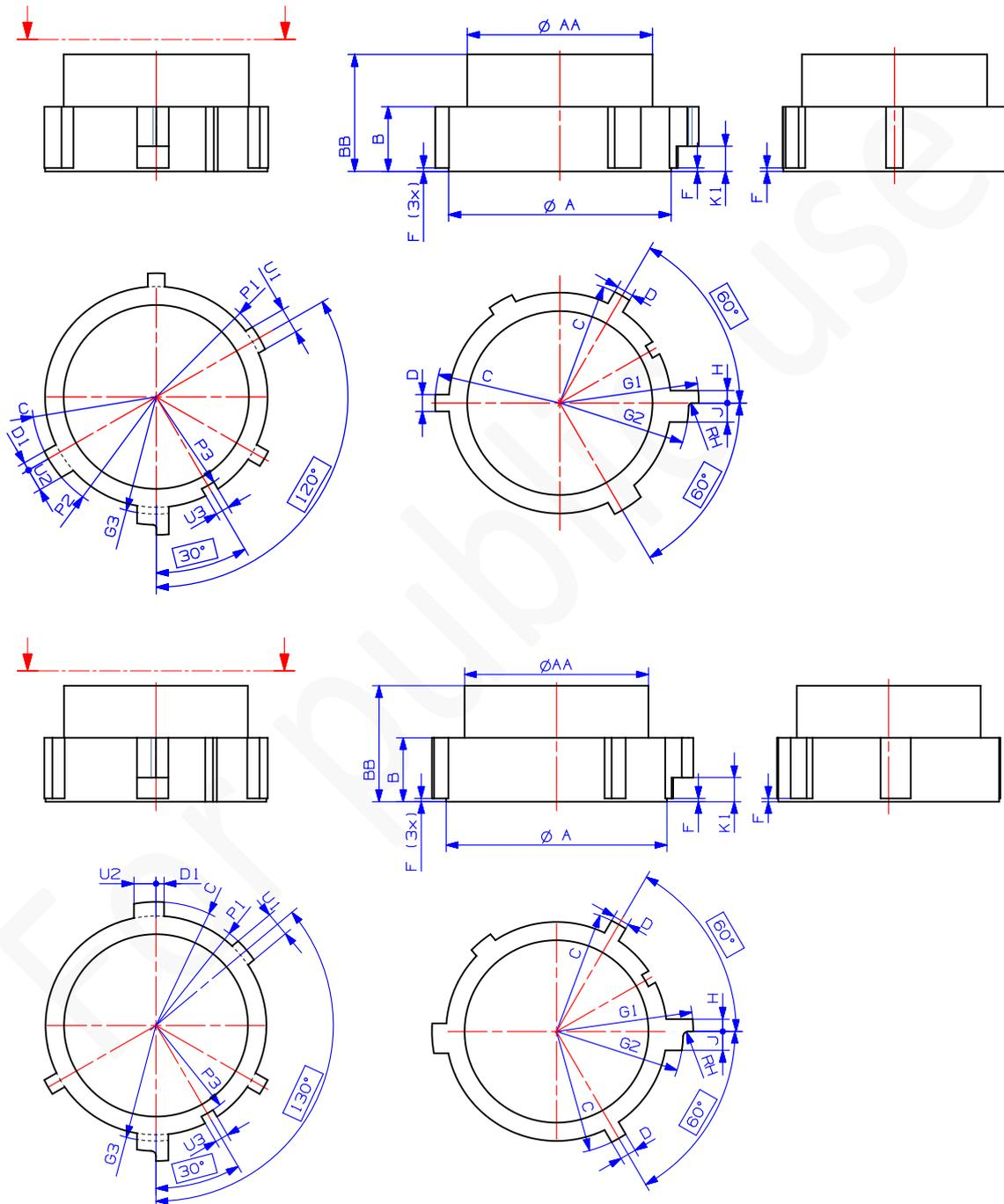
**Figure A-16 : Dimensions of MTG-H5 (top) and MTG-H6 (bottom)**
