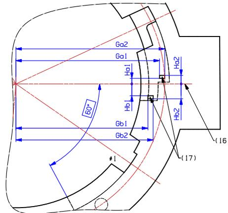
**Figure 3-7: Holder electrical contact definition**
