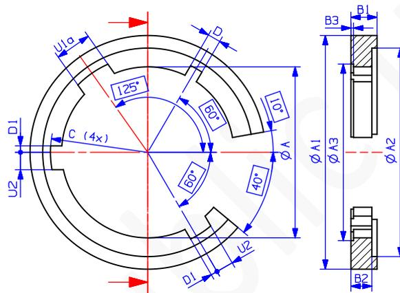
Figure A-4: Dimensions of MTG-B5a
