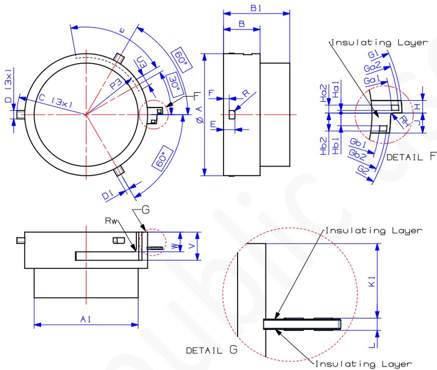
**Figure A-17 : Dimensions of MTG-H7**
