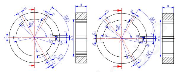
Figure A-1: Dimensions of MTG-B1 (left) and MTG-B2 (right)
