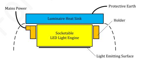
Figure 2-1: Schematic view of the assembly of a Socketable LLE, Holder and Luminaire
