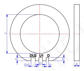
Figure A-3: Dimensions of MTG-B4
