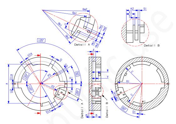
Figure A-7 : Dimensions of MTG-B6
