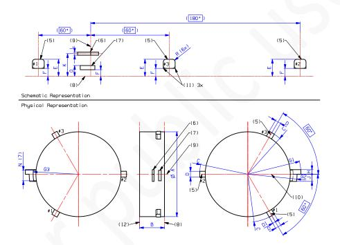
Figure 3-2: Dimensions of the Base
