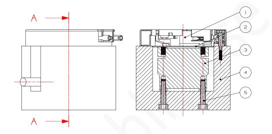
Figure A-20 : Assembly of mounting platform, force transducer and Holder under test
