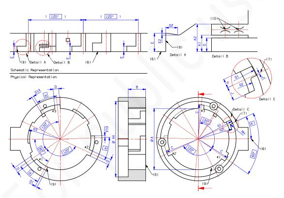
Figure 3-6: Dimensions of Holder (containing some details of a PHJ65d-1 Holder)
