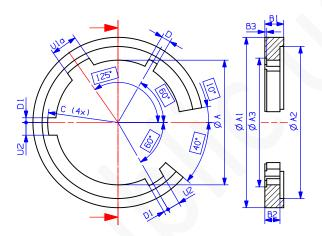
Figure A-4: Dimensions of MTG-B5a
