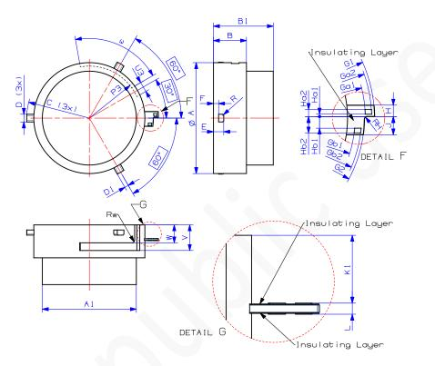
Figure A-17 : Dimensions of MTG-H7
