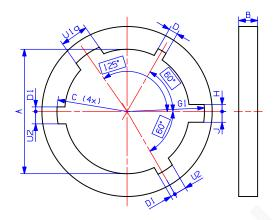
Figure A-2 : Dimensions of MTG-B3
