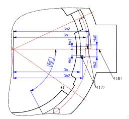
Figure 3-7: Holder electrical contact definition
