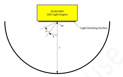
Figure 4-2: Luminous intensity distribution
