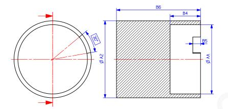
Figure A-5: Dimensions of MTG-B5b
